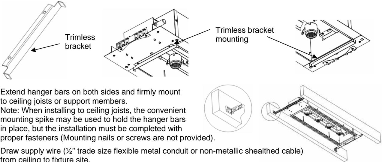
1. Extend hanger bars on both sides and firmly mount to ceiling joists or support members.
