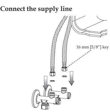
Connect the supply line. In order to guarantee a long use of the product, install the angle valve equipped with filter and clean them regularly. Do not allow the supply tube to twist or bend sharply. Flush out debris from water lines and faucet.
