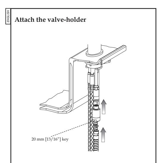
Attach the valve-holder to the shorter tubing and attach the spray hose to the valve-holder.
