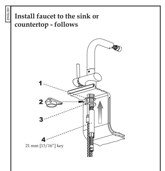
Install the fastening components to the faucet's threaded shank in the following sequence: O-ring (1), triangular flange (2), metal washer (3) and threaded nut (4) (the triangular flange can be omitted if the sink/countertop is too thick).
