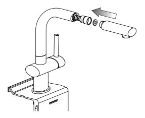
Attach the pull-out spray head to the hose. NOTE:
