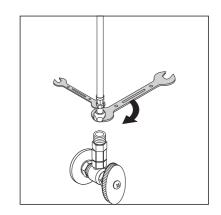
Turn on the water and check all connections for leaks.
