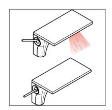
Pivot the handle to the rear for warmer water, to the front for cooler water.
