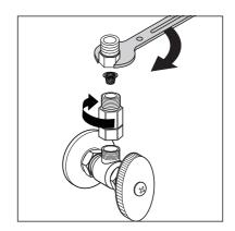
Slide the compression nut, cone washer, metal washer, and rubber washer over the end of the supply hose. Place the supply hose in the filter.
