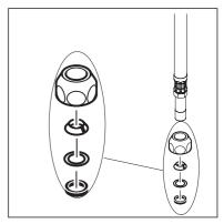
Tighten the compression nut to the filter, using two wrenches, as shown in the diagram, to prevent the supply hose from twisting.
