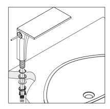
Install the adapters on the stops. Install the filters on the adapters.
