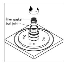
Carefully install the showerhead on the shower arm. Because of the self-sealing filter gasket, Teflon tape is normally not required.
