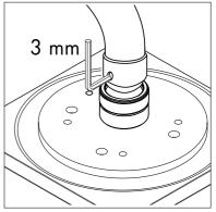
If the flow of water decreases, remove and clean the filter gasket.
