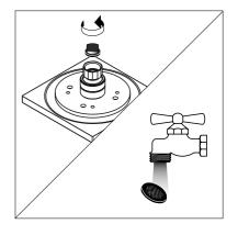
The showerhead incorporates the Rubit<sup>™</sup> cleaning system. If scale deposits are noticed in the spray channels, turn the water on lightly and rub the spray channels with a finger or a sponge.
