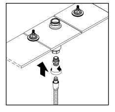
Place the handshower holder and sealing ring in the hole on the mounting surface.
