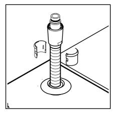
Install the hot and cold supply lines (not included).
