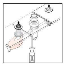
Remove the plug from the bottom of the diverter housing.
