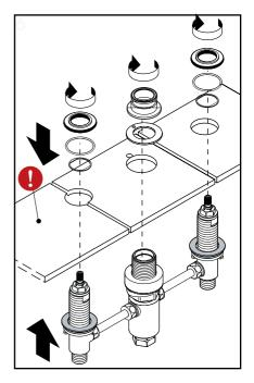
Rest the assembly on the mounting surface, with the spout adapter pin inserted in its hole.
