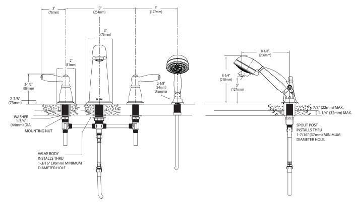
NOTE: THE INSTALLATION SHOWN IS FOR TILE DECKS, THIS VALVE WILL ALSO FIT STEEL, CAST IRON OR PLASTIC DECKS
