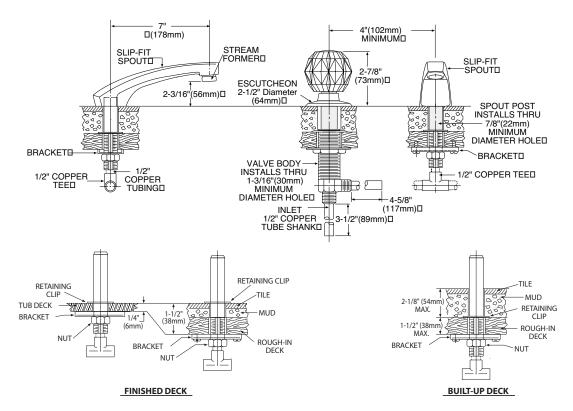
NOTE: THE INSTALLATION SHOWN IS FOR TILE DECKS, THIS VALVE WILL ALSO FIT STEEL, CAST IRON OR PLASTIC DECKS
