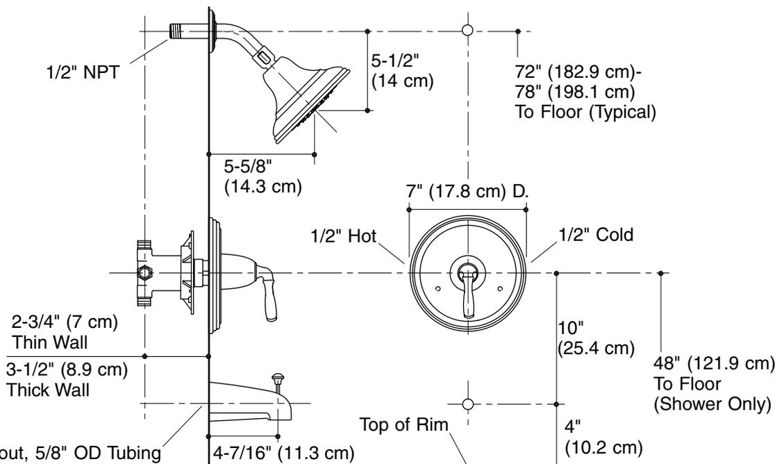
For Slip-Fit Spout, 5/8" OD Tubing Must Extend 1-1/2" (3.8 cm) Min; to 2-7/8" (7.3 cm) Max Beyond the Finished Wall.
