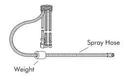
Insert the gasket into the valve outlet hose. Carefully thread the spray hose into the valve outlet hose. Tighten securely, but do not overtighten.
