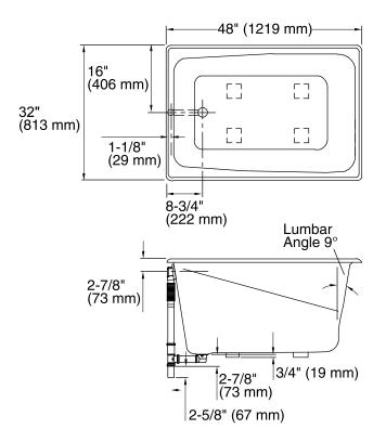
No change in measurement if connected with drain illustrated. (K-7256)
