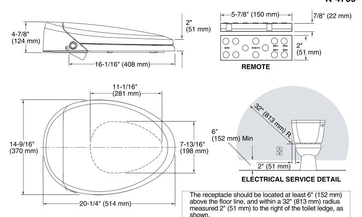
One dedicated circuit required, protected with Class A Ground-Fault Circuit-Interrupter (GFCI) or Residual Current Device (RCD).
