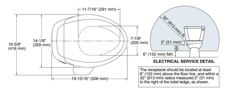
One dedicated circuit required, protected with Class A Ground-Fault Circuit-Interrupter (GFCI) or Residual Current Device (RCD).
