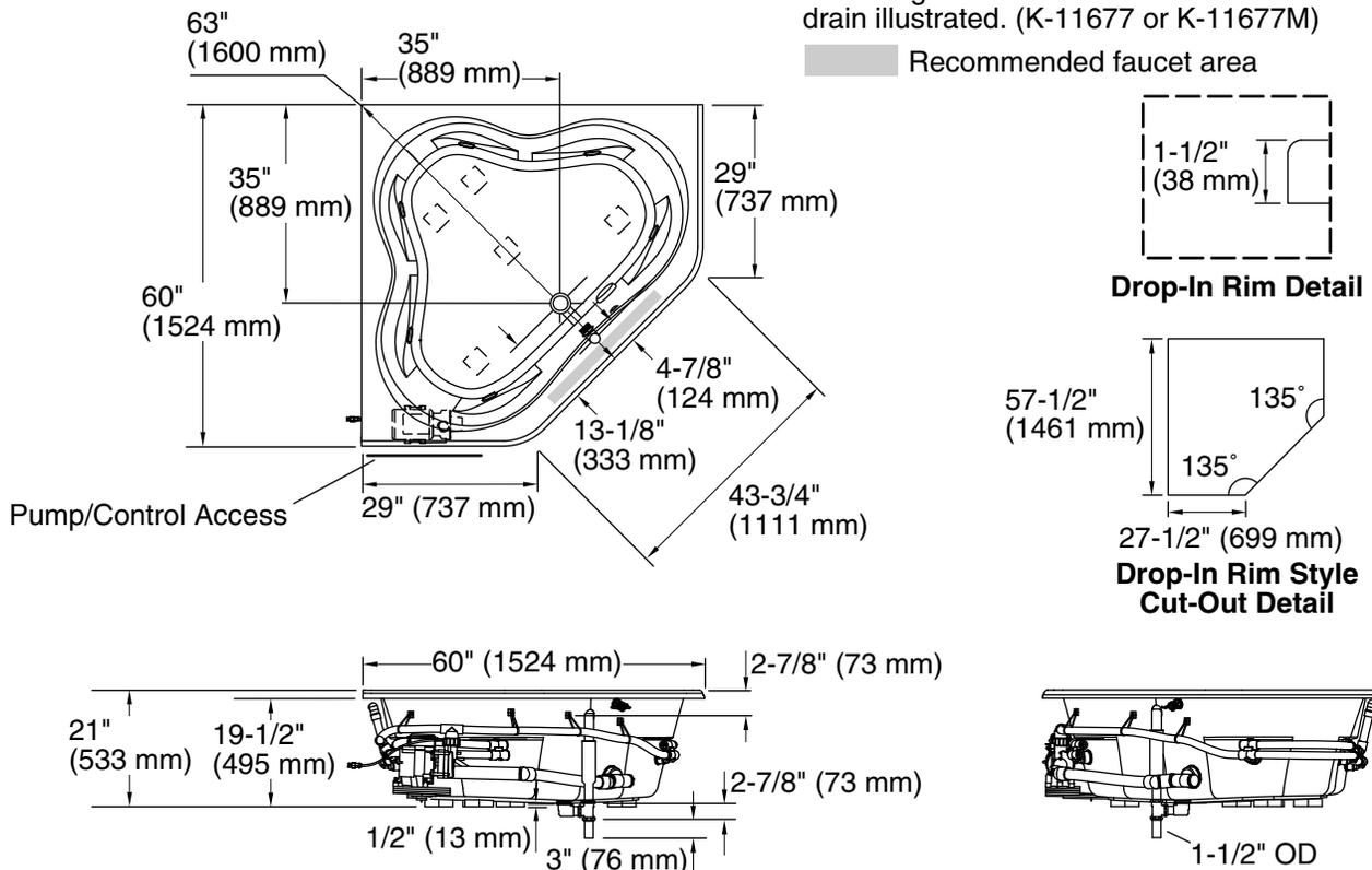
No change in measurements if connected with drain illustrated. (K-11677 or K-11677M)
