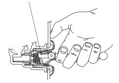
Housing Inspect and Iubricate the O-ring. Slide the O-ring onto the first shoulder of the jet.
