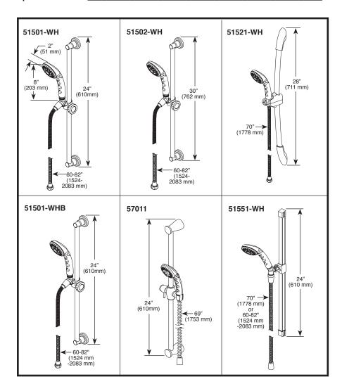
Your Delta Faucet handshower incorporates a backflow protection system that has been tested to be in compliance with ASME A112.18.3 and ASME A112.18.1/CSA B125.1. It incorporates two certified check valves in series, which operate independently and are integral, non-serviceable parts of the wand assembly.
