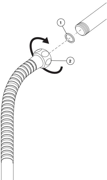
Ensure gasket (1) is inserted into the hose (2). Connect the hose to your designated water supply.
