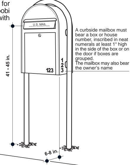
CUSTOMERS ARE REQUIRED TO CONTACT THE LOCAL POST OFFICE BEFORE INSTALLING THE MAILBOX TO ENSURE ITS CORRECT PLACEMENT AND HEIGHT AT THE STREET. GENERALLY, MAILBOXES ARE INSTALLED AT A HEIGHT OF 41–45 in. FROM THE ROAD SURFACE TO INSIDE FLOOR OF THE MAILBOX OR POINT OF MAIL ENTRY (LOCKED DESIGNS) AND ARE SET BACK 6–8 in. FROM FRONT FACE OF CURB OR ROAD EDGE TO THE MAILBOX DOOR.
