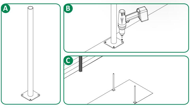
Any WamBam vinyl fence can be mounted to a wood, or concrete surface using our surface mounts.
