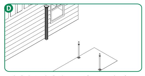
Leveling donuts can be adjusted to compensate for uneven mounting surfaces
