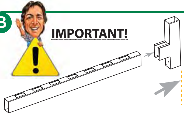
B - Insert top rail ALL THE WAY until it BOTTOMS OUT inside bracket
