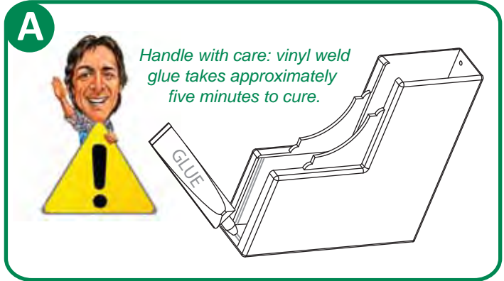
A - Run bead of vinyl weld continuously around the inside of the gate bracket
