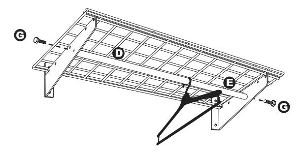
You have now completed the installation are ready to load your new HyLoft Shelf. (Maximum 150 lbs. per 18" x 36" unit, evenly distributed). Place the sticker provided on a bracket for easy access to reference information.
