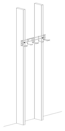
2 Both wood screws must be fastened into a vertical stud inside the wall.
