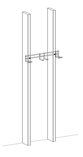
2 Both wood screws must be fastened into a vertical stud inside the wall.
