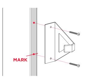
2 Mark holes through rack mounting plate, drill 1/8" pilot holes and install screws into stud. Tighten screws firmly.
