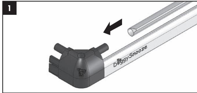
**EN** Slide the lower long frame tube onto the side of a corner. Add the upper long frame tube to the same corner. (Tear-drop edge is facing outside and downward).
