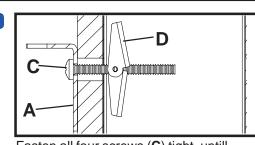
Fasten all four screws (C) tight, untill wall plate (A) is flushed with wall.
