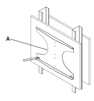
3 Drill four 3/4" (19 mm) dia. holes through drywall and studs. Insert togglers (**D**) as shown to the right...
