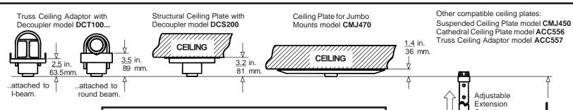
The Adjustable Extension Column for Jumbo Mounts is the most versatile choice for Jumbo Mount installations. Adjustability means that the exact position of the Jumbo Mount need not be predetermined. Length can easily be "fine tuned" at the time of installation and then locked into place.
