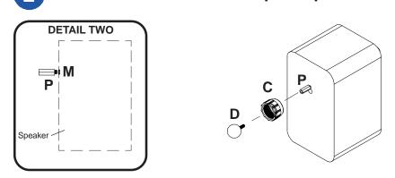
For Attachment to Speakers with a Keyhole on Back: Thread keyhole adapter (M) into coupling (P) a few turns. Insert assembly into keyhole on back of speaker as shown in DETAIL TWO. Hand tighten coupling (P) until it fits tightly against back of speaker. Use 7/16" open end wrench to tighten coupling (P) until it is secured to speaker. Insert ball (D) through cap (C) and thread into coupling (P). Hand tighten ball (D) until it is secured to coupling (P).
