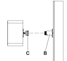
Thread ball/cap assembly onto mounting base (**A**) or extension (**B**) by hand. For heavier speakers, it may be necessary to tighten cap (**C**) with channel locks. If so, wrap a cloth around cap (**C**) to prevent damage.
