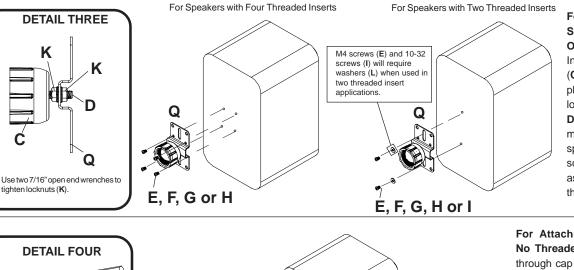
For Attachment to Speakers with More Than One Threaded Insert: Insert ball (D) through cap (C) and attach mounting plate (Q) using two serrated locknuts (K) as shown in DETAIL THREE. Attach mounting plate (Q) to speaker using two or four screws (E),(F),(G),(H) or (I) as needed for speaker threaded insert pattern.
