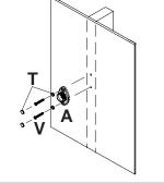
For Attachment to Wood Stud Walls: Use a stud finder to locate center of stud. Drill two 3/16" (5 mm) dia. holes to a minimum depth of 2" (51 mm). Attach mounting base unit (A) to center of wood stud using two wood screws (V) and two plastic screw plugs (T) as shown left.
