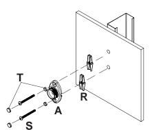
For Attachment to Metal Stud Walls or Direct Attachment to Drywall for Speakers Over 10 lb: Use a stud finder to locate center of stud. Drill two 5/8" (16 mm) dia. holes through metal stud. Attach mounting base unit (A) to center of metal stud using two #10-24 phillips screws (S), two plastic screw plugs (T) and two togglers (R) as shown in DETAIL ONE.
