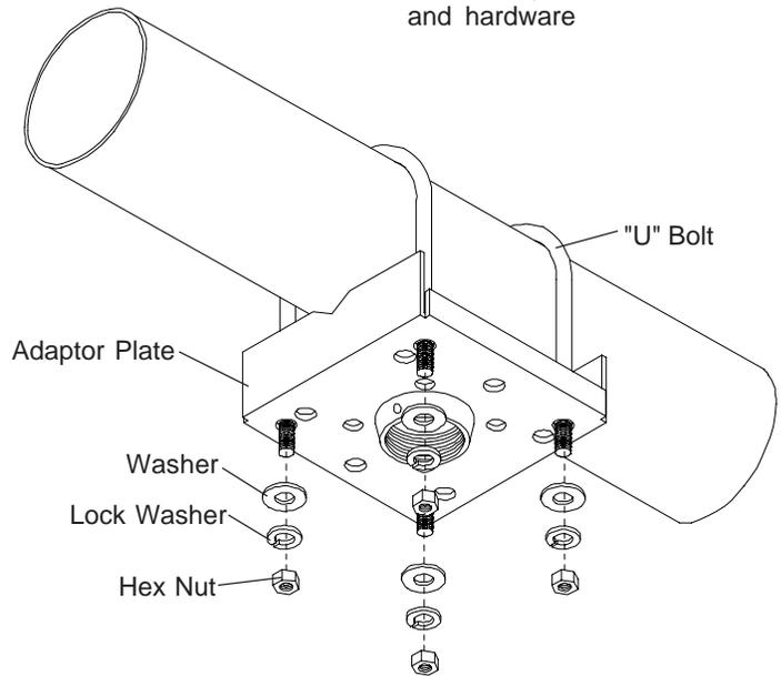
**Note:** Insert the M5 x 10 mm tri-point screw in the threaded pipe fitting as directed in the extension column instructions. If you are using an extension pipe without a notch, drill a 11/64 (0.172") dia. hole through the pipe and insert the screw through the pipe. **Failure to do so could cause the assembly to fail.**
