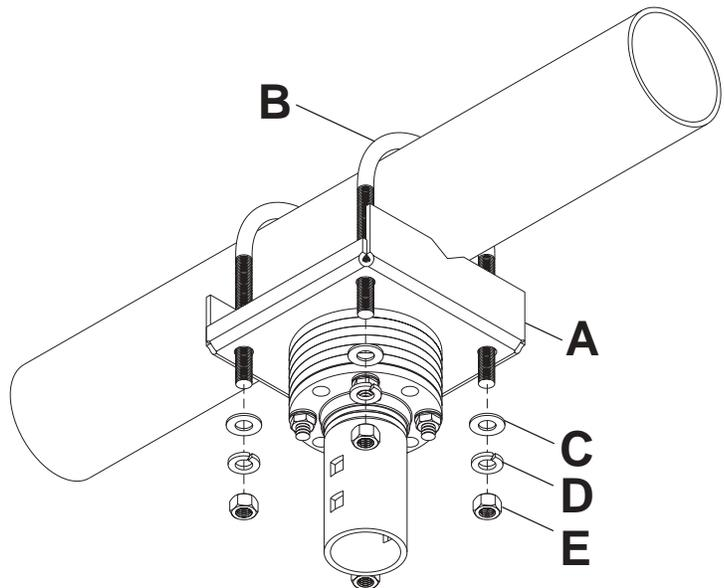
**Detail 1** The orientation of the decoupler assembly will depend on the shape of the truss
