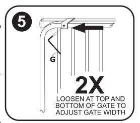
Use Allen wrench (G) to unscrew set screws on top and bottom of gate to extend gate. LEAVE SHIPPING TABS IN PLACE TO NOT MAR GATE FINISH. You will remove shipping tabs during final tightening.
