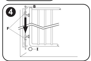
Hang gate by inserting hinge rod ( $\bf B$ ), through top of mounted hinge bracket ( $\bf A$ ), through upper plastic shoulder washer ( $\bf F$ ), through both eye bolts, through 4. lower plastic shoulder washer (**F**), and finally through bottom of hinge bracket. To secure hinge, insert key ring (I) through hole in end of hinge rod. Gate can be mounted at angles up to 30 degrees.
