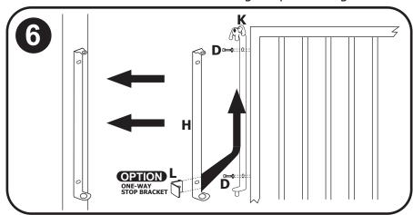
Mount latch assembly (**K**) to gate using 3/4" bolts with serrated washers (**D**). Attach wall mount for latch assembly (**H**) up into part (**K**) that is now secure on gate. Slide gate out to mark holes for (**K**) on attaching wall. (\*OPTIONAL ONE WAY BRACKET INSTALLED HERE) Then attach the wall mount of latch assembly to wall using Phillips head screws (**C**). Optional long screws (**j**) maybe be used to attach gate to stud through dry wall.
