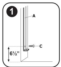
1. Install hinge bracket (A) to wall (stationary side of gate) using Phillips screw (**C**) beginning 6½" above floor surface.
