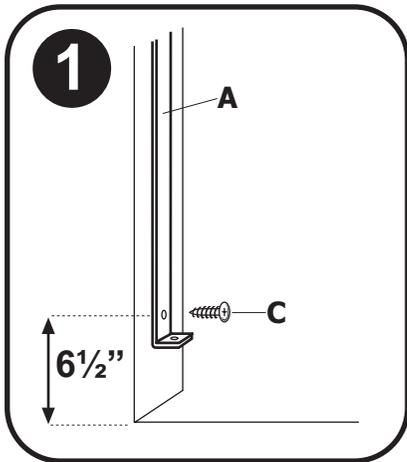
**1.** Install hinge bracket (A) to wall (stationary side of gate) using Phillips screw (C) beginning 6 1/2" above floor surface.
