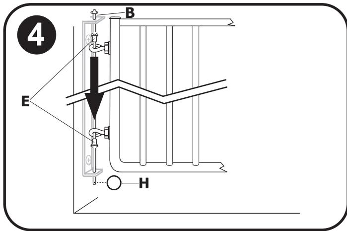
**4.** Hang gate by inserting hinge rod (B), through top of mounted hinge bracket (A), through upper plastic shoulder washer (E), through both eye bolts, through lower plastic shoulder washer (E), and finally through bottom of hinge bracket. To secure hinge, insert key ring (H) through hole in end of hinge rod.
