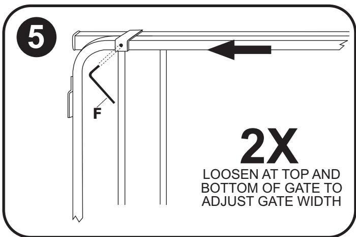
**5.** Use Allen wrench (F) to unscrew set screws on top and bottom of gate to extend gate to fill door opening. ONLY LIGHTLY TIGHTEN AND LEAVE SHIPPING TABS IN PLACE NOT TO MAR GATE FINISH. You will remove shipping tabs during final tightening.
