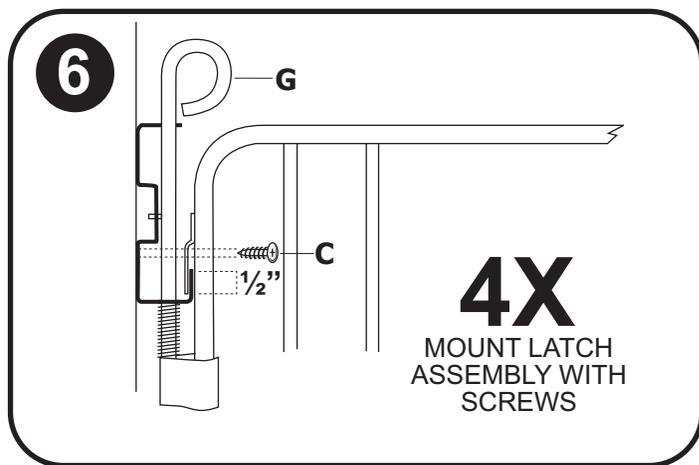
**6.** Hold latch assembly (G) against opposite wall and extend gate until at least 1/2" of safety bracket will interlock with flange of latch. Mark position of latch assembly screw holes with pencil. Swing gate out of way and mount latch assembly to wall. Check closure of gate and tighten set screws from STEP 5 by removing shipping tabs to secure gate width.
