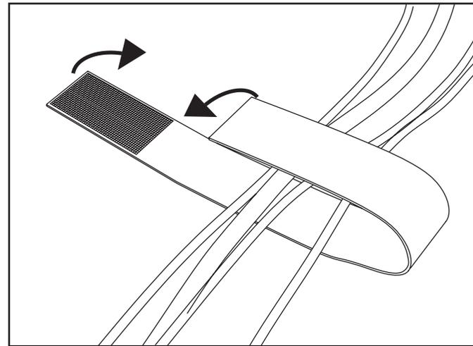
Wrap wires with soft side of strap facing out.
