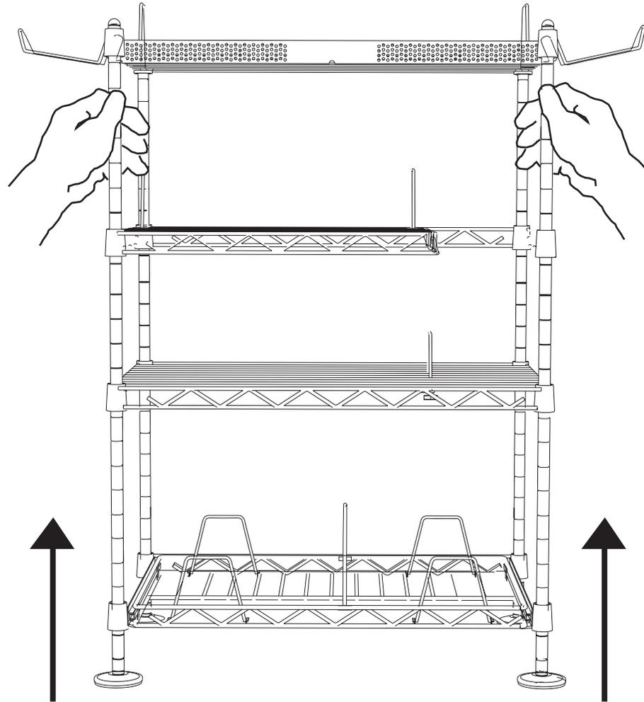
To move unit: Hold onto rods and carefully lift. **DO NOT** hold or lift with the shelves
