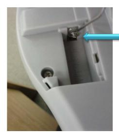
Locate the spring which is underneath 2 plastic "sides" and use an open paperclip to gently pull the spring forward in front of the plastic sides. Do the same thing for both side slots where batteries go. The batteries will now make a connection.
