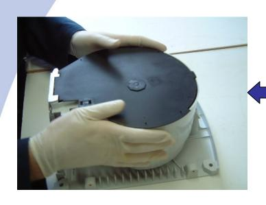
Step 2: Remove the fan wheel by unscrewing the center nut.
