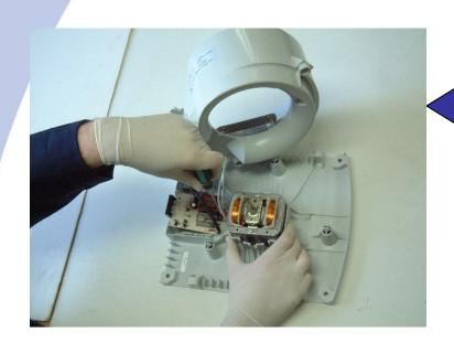
Step 6: Disconnect the two cables of the heating element (the white ones) from the circuit board.
