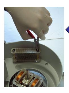
Step 3: Remove the clips on the upper part of the heating element.
