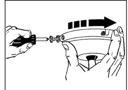
Rotate canopy clockwise until both mounting scréws drop into slot recesses. Tighten screws securely. Install third and fourth screws with lockwashers into mating holes and tighten.
