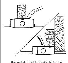
Use metal outlet box suitable for fan support. Secure outlet box directly to the building structure using ceiling joist screws (included). Junction box must support 35 lbs
