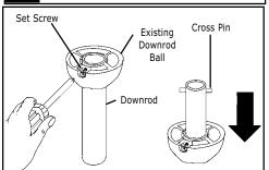
Remove the downrod ball that was supplied with your ceiling fan by loosening the set screw on the side of the ball so that it is no longer making contact with the downrod. Slide the downrod ball off the downrod. Be sure to keep the
