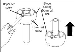
With your new longer downrod or your existing downrod, install the Slope Ceiling
