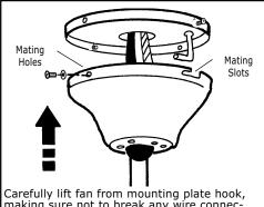
making sure not to break any wire connections. The canopy has (2) mating slots and (2) mating holes (see illustration above). Position both slots in canopy directly under and in line with (2) mounting plate screws and lock washers. Lift fan
