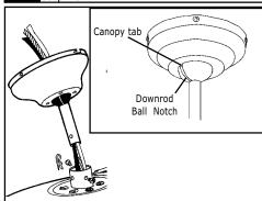
Feed motor lead wires through downrod/ canopy assembly and insert downrod into motor yoke. Make sure that the tab in the canopy engages the notch in the downrod
