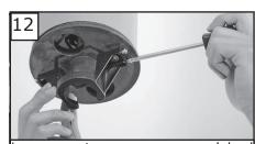
Loosen two preassembled screws across from each other corresponding to the open slotted holes on the canopy upper rim and remove the other two screws from mounting bracket. Keep screws for later use.
