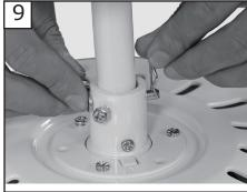
Insert downrod into the yoke on top of fan body. Align the hole in the downrod with the hole in the yoke. Insert cross pin through yoke and downrod until point appears on the other side.
