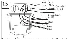
Make wiring connections as indicated above. Connect black and blue wire from fan to Black or (Hot) wire from house. Connect White wire from Fan to White (Neutral) wire from house. Connect Ground leads from mounting bracket and downrod to Ground lead from house. Refer to Safety Tips section of manual.
