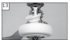
Hang assembled fan from the mounting bracket installed to ceiling in previous step. Make sure the fan is hanging straight. Rotate fan until the tab on the Mounting bracket engages the slot on the Downrod Ball. This must be done to prevent the fan body from rotating when the blades are in motion.
