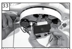
Attach capacitor onto switch housing by preadhered double-sided foam tap as shown.
