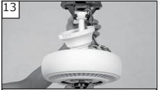
Hang assembled fan from the mounting bracket installed to ceiling in previous step. Make sure the fan is hanging straight. Rotate fan until the tab on the Mounting bracket engages the slot on the Downrod Ball. This must be done to prevent the fan body from rotating when the blades are in motion.
