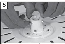
Remove keeper pin and cross pin from yoke, and save for later use.
