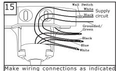
above. Connect black and blue wire from fan to Black or (Hot) wire from house. Connect White wire from Fan to White (Neutral) wire from house. Connect Ground leads from mounting bracket and downrod to Ground lead from house. Refer to Safety Tips section of manual.
