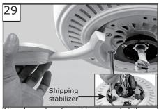
Check motor for shipping stabilizers and remove if present. Install the blade assembly to motor using the screws pre-installed. Tighten screws securely. Repeat this process for remaining blade assemblies.
