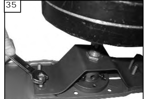
35 The studs on the mounting plate protrude through the slots in the motor bracket. Securely tighten the locknuts onto the threaded studs.
