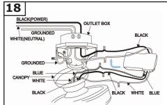
Make wiring connections as indicated above. White from fan to white from remote marked N. Blue from fan to blue from remote marked light. Black from fan to Black from remote marked L. White from house to white from re-mote marked AC N . Black from house to Black from remote marked AC L. Connect all green ground wires to Grounded wire from House.
