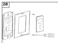
Attach front cover to wall control with screws provided. Snap battery cover in place.
