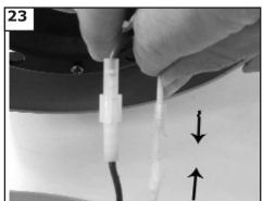
Connect white wire from fan to White wire from light fixture. Connect blue wire from fan to Black wire from light fixture.
