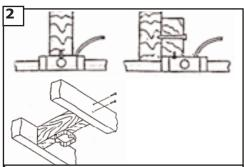
Before installing this fan make sure the outlet box is properly installed to the house structure. To reduce the risk of fire, electric shock, or personal injury, mount to outlet box or supporting system acceptable for fan support. (Mounting must support at least 35 lbs.)
