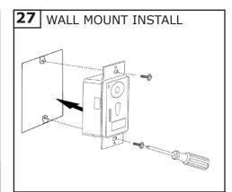
Install wall control unit to outlet box using machine screws provided.
