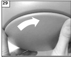
Attach blanking plate by locating dimples in light fixture with grooves in the blanking plate and twist clockwise.
