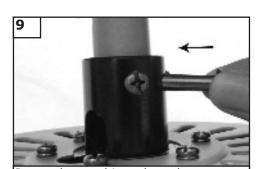
Insert downrod into the yoke on top of fan body. Align the hole in the downrod with the hole in the yoke. Insert cotter pin through yoke and downrod until point appears on the other side
