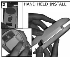
Place face plate over battery compartment and buttons. Place remote over 2 pins on front cover. Attach cover of remote by placing over 4 pins and snaping into place.
