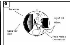
Align gap in receiver with the screw between speed switch and reverse switch and slide receiver (Dip switch facing housing plate) into switch housing plate. Receiver should fit directly into area in the switch housing plate. Note: If installing light kit, use the blue and white wire from the receiver.
