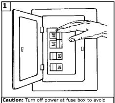
**Caution:** Turn off power at fuse box to avoid possible electrical shock.
