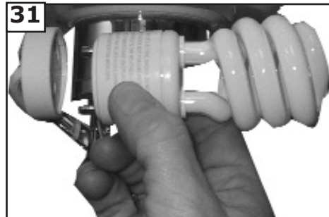
Install 2 x 13 watt GU24 base CFL bulbs. Bulbs Included. WARNING: Over lamping the fan will result in the fan lights shutting down until the proper wattage of bulbs are installed. Reset the lights by turning off the wall switch, breaker, or by remote. Replace bulbs with the correct wattage bulbs, turn the power on.
