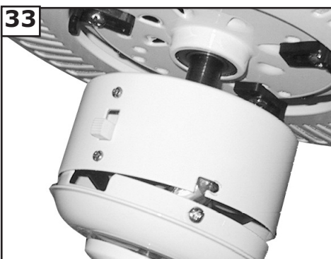
Attach switch cap to fan by lining up 2 slot ear holes and 1 screw hole and twisting cap. Then tighten the 3 screws.
