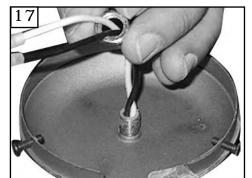
Install keeper nut over lead wires.
