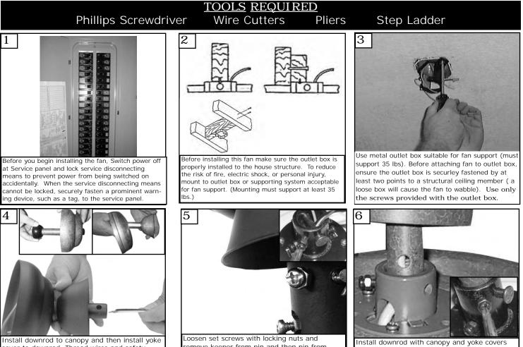
Install downrod to canopy and then install yoke cover to downrod. Thread wires and safety cable through downrod Loosen set screws with locking nuts and remove keeper from pin and then pin from yoke for downrod (see inset).
