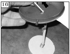
Install switch housing to light kit by turning clockwise to tighten.
