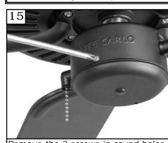
Remove the 3 screws in round holes. Remove cap by twisting and pulling down. Save screws.
