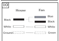
Connect black and blue wire from fan to Black or (Hot) wire from house. Connect White wire from Fan to White (Neutral) wire from house. Connect Ground leads from mounting bracket and downrod to Ground lead from house. Refer to Safety Tips section of manual.
