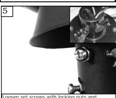
Loosen set screws with locking nuts and remove keeper from pin and then pin from yoke for downrod (see inset).
