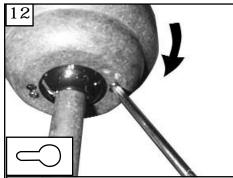
Lift canopy to ceiling aligning the key hole slots with the screws on the bottom of the mounting bracket. Rotate the canopy counter clockwise to lock in place. Tighten the screws to secure the canopy. See insert for key hole shape.
