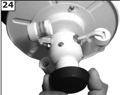
24 Remove the finial cap, hex nut, and rubber pad from the fitter.
