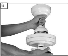
Carefully lift fan assembly onto mounting bracket. Rotate fan so that the notch on the ball engages the ridge in the mounting bracket. This will allow hands-free wiring.
