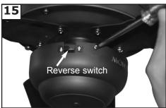
Install the switch housing using the 3 screws previously removed. Setting the reverse switch in the left hand side will result in downward airflow and setting the switch in the right hand side will result in upward airflow.
