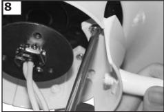
Remove 2 screws per blade holder. Remove blade holder. When replacing blade holders make sure the screws are tightened securely to the motor.
