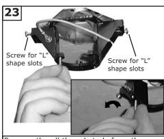
Remove the all thread studs from the lower part of the mounting bracket. Install 2 screws that align with the "L" shape holes in the canopy into the mounting bracket. (see step 15)
