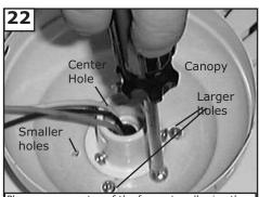
Place canopy on top of the fan motor allowing the yoke to pass through the large hole in the center of the canopy. Align the 3 larger holes around the center hole with the 3 screws already installed in the fan. Install 3 flush mount screws removed previous step into smaller holes and tighten securely.
