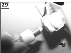
install 1 x 100 watt halogen bulb with socket type E-11. Do not touch bulb surface as oily residue from skin can cause the bulb to explode.
