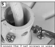
Loosen the 2 set screws in yoke for downrod to slip into yoke.
