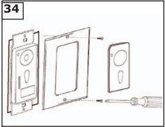
Attach front cover to wall control with screws provided. Snap battery cover in place.
