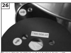
Swing blade holders out and align hole with arrow on blade holder with hole in blade with arrow. Make sure that the side of the blade that has the sticker this side up is facing upward.
