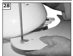
Tighen screws securely. Repeat this process 4 more times until all blades are assembled.
