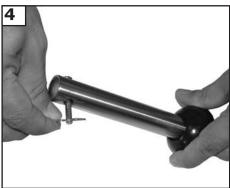
Remove keeper from pin. Put keeper back in pin and save for later.
