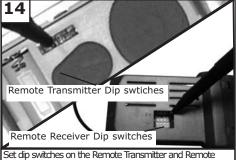
Set dip switches on the Remote Transmitter and Remote Receiver to the same settings. This must be done so the units will communcate properly. If you have other fans you can set to control from one transmitter by setting both receivers the same as the transmitter. If you have more than one fan with remote. You can set the dip switches to different positions to have seperate control.
