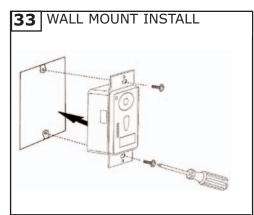
Install wall control unit to outlet box using machine screws provided.
