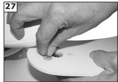
Install 3 screws and fiber washers to back side of blade as shown.
