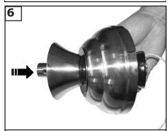
Place canopy, canopy disk, yoke on downrod as in photo. Then thread leadwires and safety cable through the downrod in direction of arrow.
