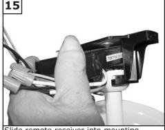
Slide remote receiver into mounting bracket.
