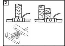
Before installing this fan make sure the outlet box is properly installed to the house structure. To reduce the risk of fire, electric shock, or personal injury, mount to outlet box or supporting system acceptable for fan support. (Mounting must support at least 35 lbs.)
