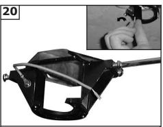
Take 4 screws from hardware pack and insert 2 one on each side of bracket to match the L slot screw holes in canopy. Keep 2 screws for later use. Remove the all thread studs from the lower part of the mounting bracket.
