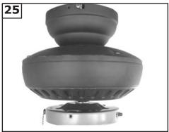
Lift fan to mounting bracket, aligning the "L" shape holes with the scresws on the mounting bracket. Turn the fan clockwise to lock in position. Install the screws that were not installed from earlier step. Tighten securely.
