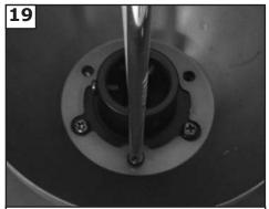
Replace the 3 screws removed and tighten securely. Check motor for shipping stabilizers and remove if present.
