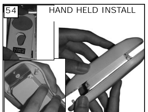
54 HAND HELD INSTALL Place face plate over battery compartment and buttons. Place remote over 2 pins on front cover. Attach cover of remote by placing over 4 pins and snapping into place.
