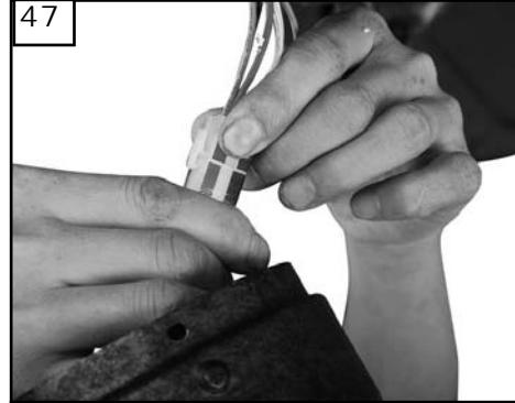
47 Plug connector from fan to connector from switch housing.
