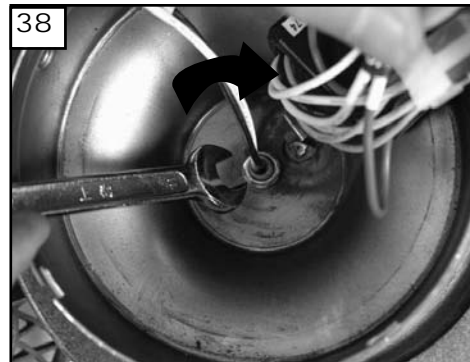
38 Install lockwasher and hex nut provided and tighten securely.
