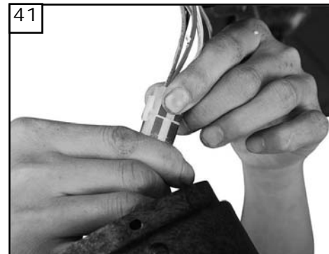
41 Plug connector from fan to connector from switch housing.
