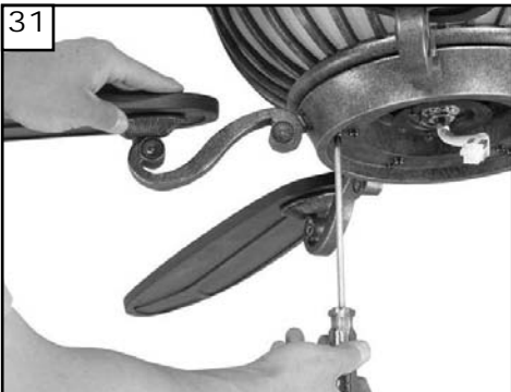
31 Attach blades to motor and tighten screws securely using screws, washers and motor pads in hardware packs.
