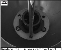
Replace the 3 screws removed and tighten securely. Check motor for shipping stabilizers and remove if present.
