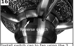
Install switch cap to fan using the 3 screws provided. Tighten securely. Setting the reverse switch in the left hand side will result in downward airflow and setting the switch in the right hand side will result in upward airflow.
